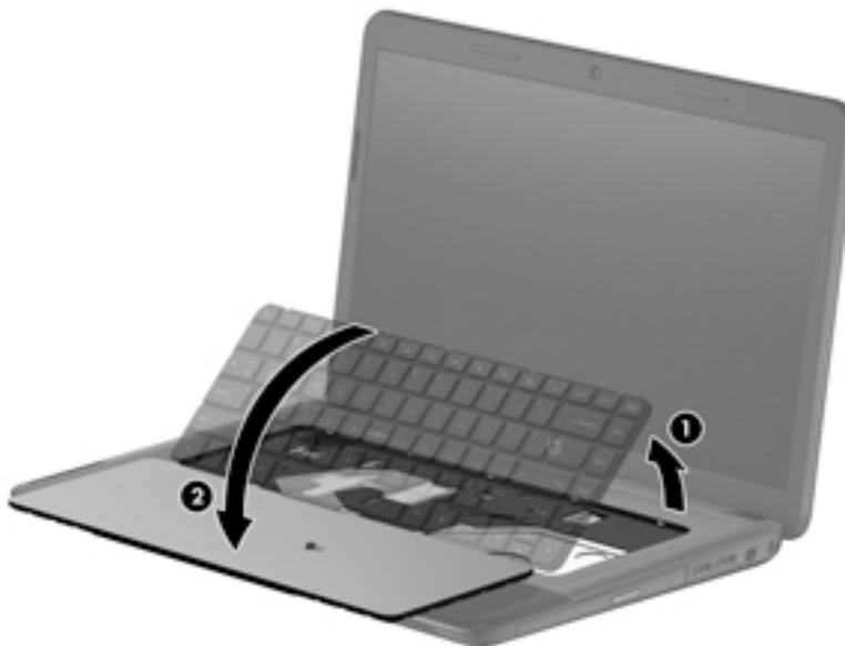
7. Release the ZIF connector **(1)** by lifting the connector tab to which the keyboard cable is connected, and then disconnect the keyboard cable **(2)** from the system board.
